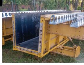
The all-steel, three-piece beams with welded in-place chamfer are easily assembled to accommodate a variety of depths and widths.
